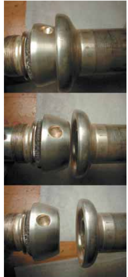
Fig 9a Contacts shown in Closed-Arc starting step-Opened position
