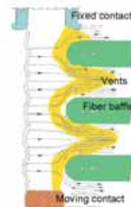
Fig 3 Representation of electric arc in oil circuit breaker
