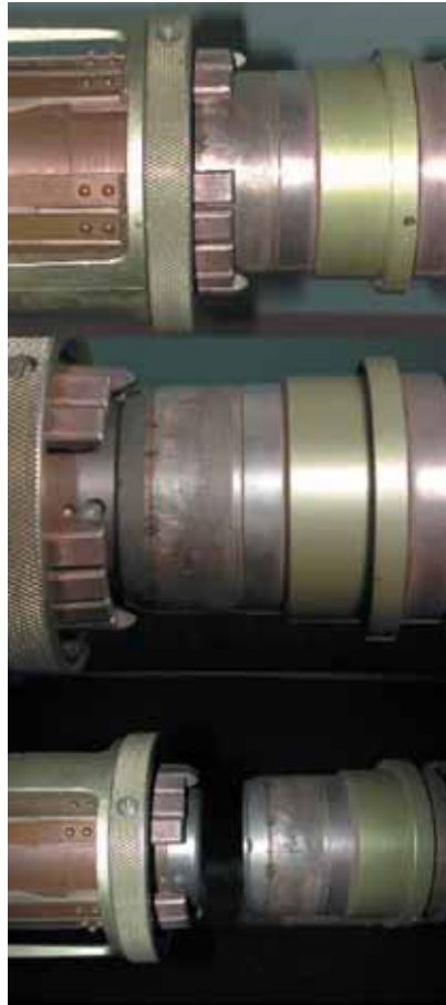
Fig 8b Contacts shown in Closed-Arc starting step-Opened position
