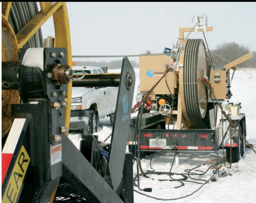
AFS303 Hydraulic controls help eliminate conductor galloping and offer smooth speed variation.
