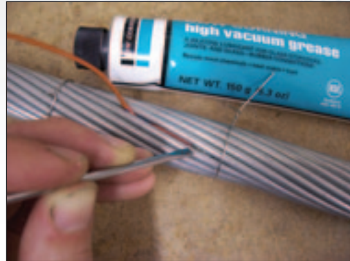
Attaching a thermocouple under the outer layer
