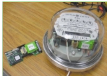
Figure 2: The AMR module shown at left is mounted under the meter disk and provides auto dial capability to send interval load data to UDRI/MeterSmart, the outside data services provider under contract to Sharyland Utilities.
