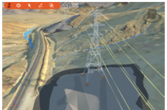
3D model of proposed 220 kV tower with footing and conductor on proposed grading limit and new roads.
