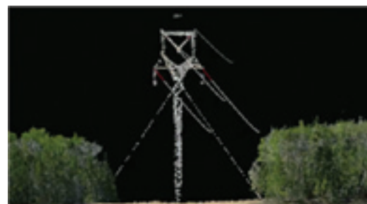
PLS-CADD Model is stripped of legacy LiDAR data on vegetation and up to date studies on refreshed data completed.
