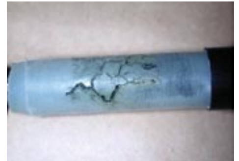
Figure 14. Poor Workmanship Leads to Failure in Pre-molded Splice Installation
