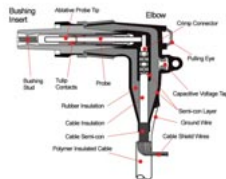
Figure 13. Elbow and Bushing Insert Drawing
