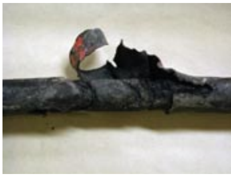
Figure 11. Cable failing from the outside in
