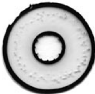
Figure 8. Cable wafer with extensive voids
