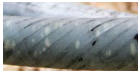
Figure 10. XLPE cable with a forest of water trees
