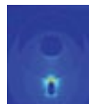
Figure 6. E-Field Color Contour Plot - No Insulation Shield near metal point.
