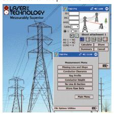
Collecting measurements safely can be directly related to LTI's reflectorless technology. Field crews no longer have to physically climb a tower or extend a height stick to a wire to obtain the measurements they need. LTI lasers have the ability to measure directly to the conductor without the need of any reflectors; therefore field crews do not have to occupy any dangerous areas.
