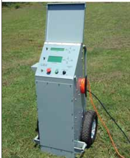
VLF Cable Testing
