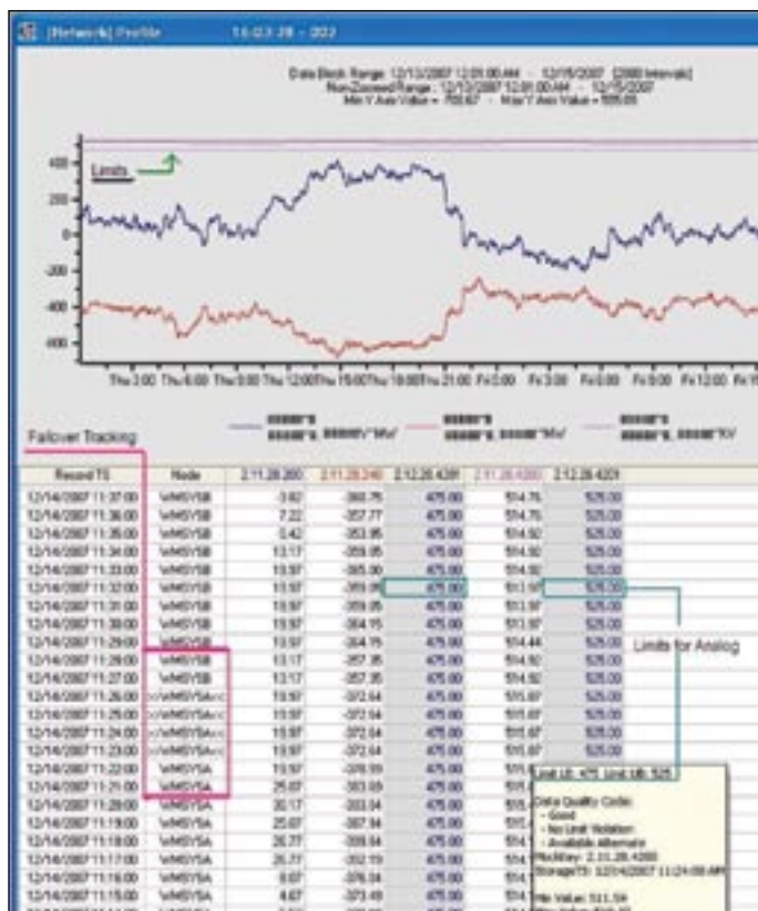
Figure 2: SCADA measurements are tightly integrated with the EMS information, including the enabled host, limit pair(s), quality codes and system alarms. The screenshot shows a typical system failover from node WMSYSA ("System A") to WMSYSB ("System B"), identifying data captured where neither node is enabled with the symbols ">> <<". Also shown are the actual limit values for one of the displayed analogs.
