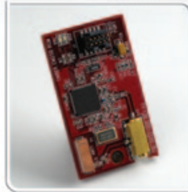
Typical ZigBee Radio Module (with internal antenna and external connectors)
