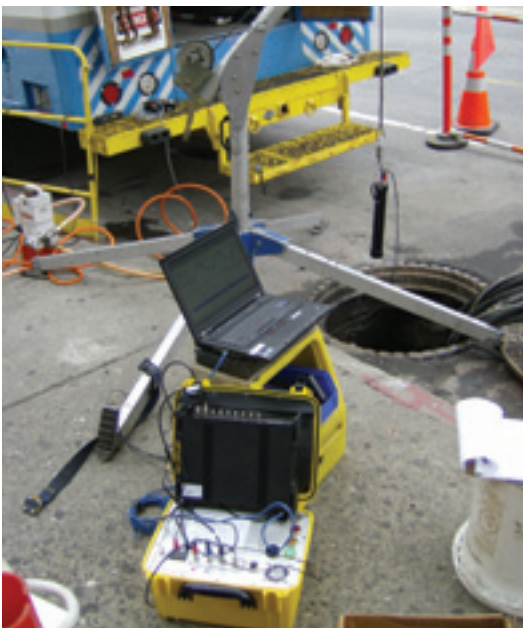
MARS device sensor pod readied for lowering into a manhole during field testing
