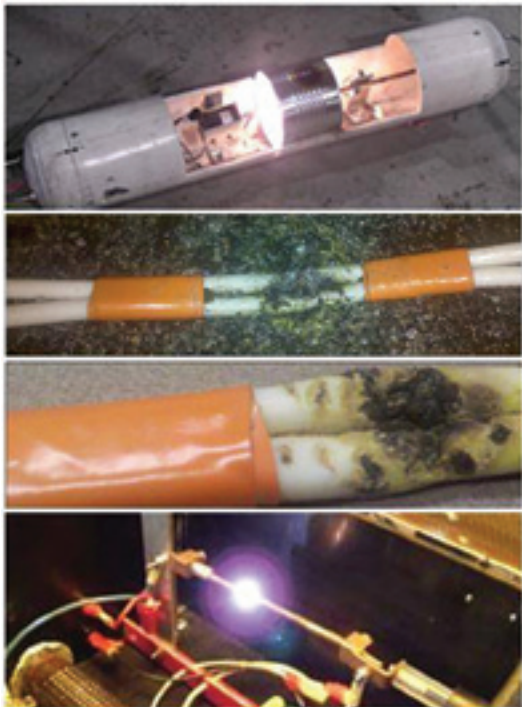
Figure 1: Example Arc Sources from Preliminary Lab Tests
