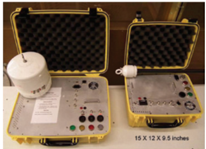
Figure 3: The first prototype MARS systems focused on size and cost reduction.
