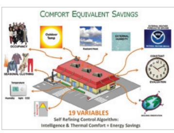
In order to ensure the maximum reduction in energy consumption, while still providing a comfortable climate, building control systems must take a wide range of factors for controlling the HVAC system into account.
