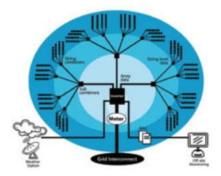
**Figure 1**. System performance is monitored at the string level, and this data is used to identify wiring, shading, or other minor maintenance issues that might otherwise escape detection.
