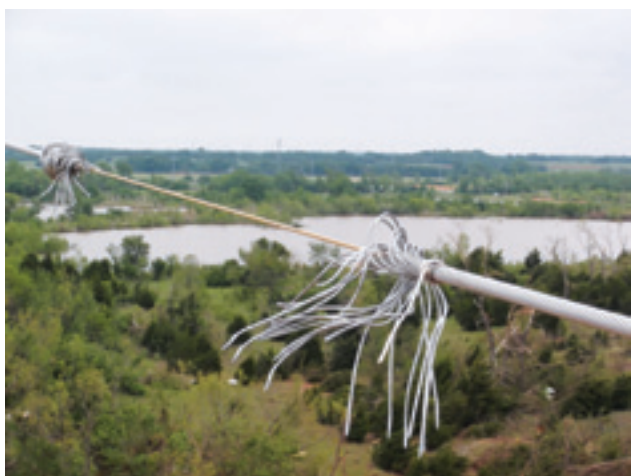
Storm damage – ACCC core remained undamaged
